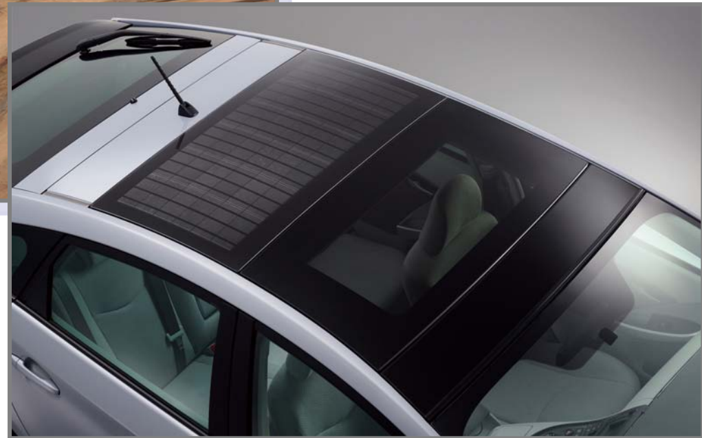
PV roof, TOYOTA Prius
